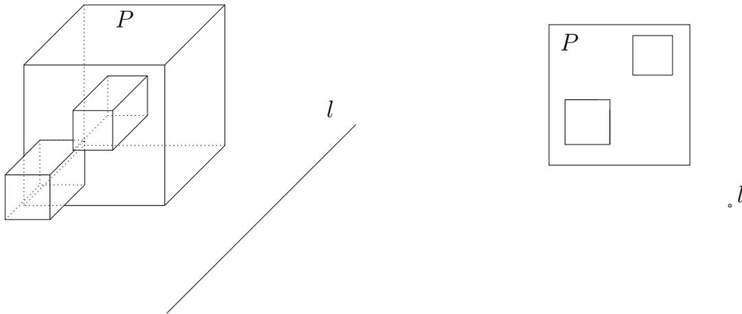
Figure 4: Example of polyhedron  $P$  that is not castable with respect to  $l$  although  $l$  does not intersect the black regions induced by  $P$ . Figure shows perspective view and front view.
